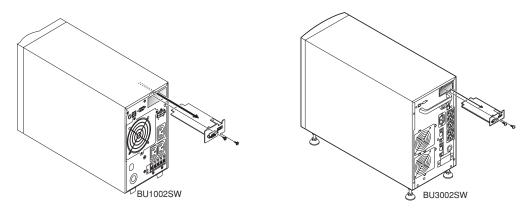
(2) Carefully insert the SNMP/Web card (model number: SC20G), and securely tighten the 2 screws. \* Replace with BU50SW/BU75SW/BU100SW/BU150SW/BU1002SW/BU3002SW brackets.
